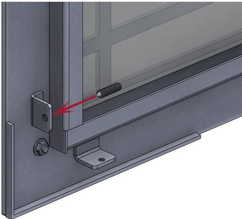
3. Insert the Pressure Screws (A) into the threaded holes on the pressure tabs.
