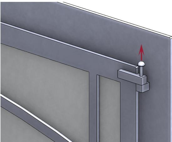
1. Remove the Glass Doors from the Main Frame. If the hinges have hinge pins, remove them first. Then lift up on the doors, lifting them off of their hinges.
