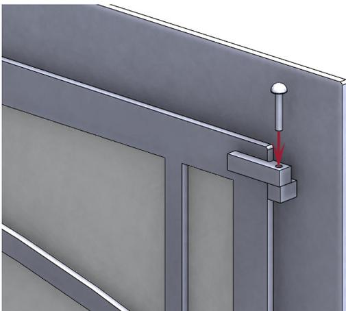
7. Re-install the Glass Doors. If your door has temporary plastic shipping hinge screws, discard them at this time and install the metal hinge pins that are taped to the glass doors (if applicable). *NOTE: Some door styles use hinges that do not use separate hinge pins.*
