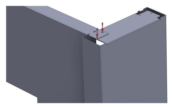
Attach the rear mounting bracket (e) to the top of the vertical supports. Insert the cleats through the corresponding slots, and secure in place with the provided self-tapping screws.
