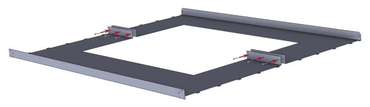
Standing the face panels upright, connect both vertical supports (c) to the face panels through the appropriate slots. (Each vertical support has lasercut slots cut that correspond with cleats on the face panels). Using a rubber mallet, ensure cleats are fully seated in the corresponding slots.
