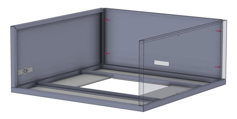
Once all of the panels have been installed, insert 2 of the corner brackets into the remaining section, and fasten in place as shown.
